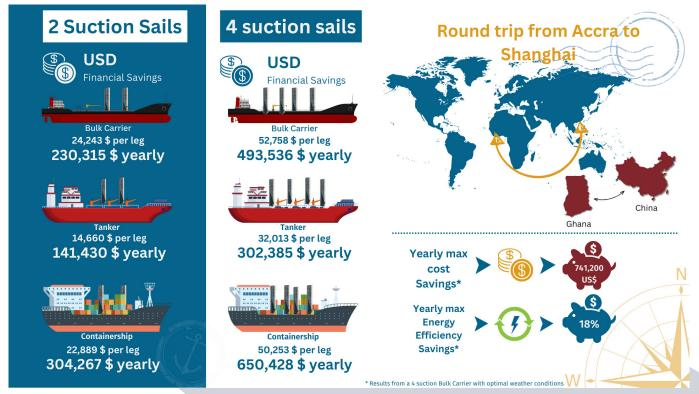
While containerships see the total greatest CO2 reduction and money savings on this model, it is important to note that 30m suction sails on the deck of a containership, would in practice negatively affect the aerodynamics, or if raised on a stub mast could interfere with port operations. These interactions need to be further researched.
