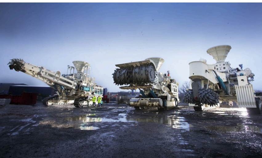
Extractor vehicles developed for the Bismarck sea by the bankrupted DSM company Nautilus Minerals. Photo by engineering company SMD.
